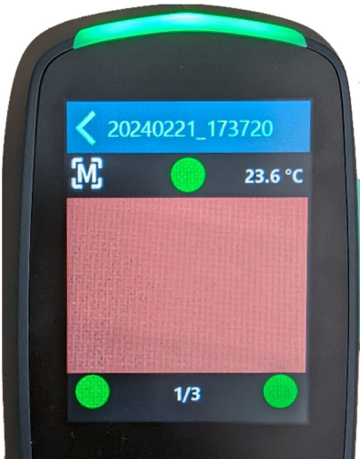
Example 1: All contact sensors are contacting correctly, and a measurement can be triggered
