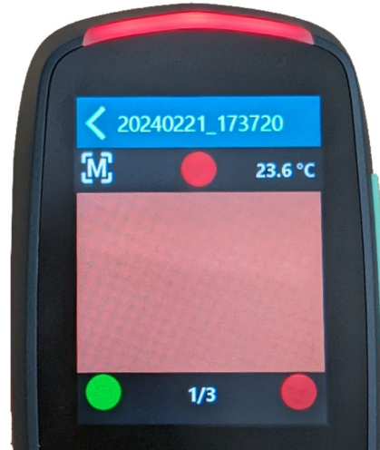
Example 2: Two contact sensors are not contacting, and the measurement cannot be triggered
